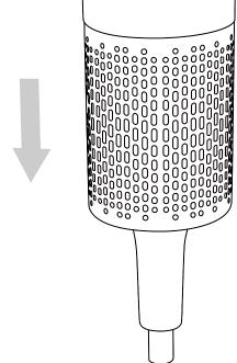
2. Remove dust or debris from the filter cover and filter net with a soft brush or lint-free cloth. (Do not clean the filter with water; Do not apply large pressure to the filter.)
